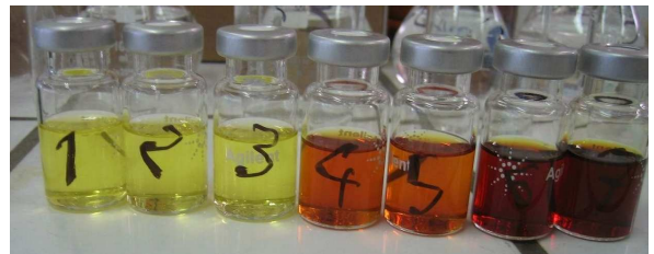
Quick test for water content : samples 4 to 8 are OK (< 750 ppm water), samples 1 to 3 are not OK (> 750 ppm water)
